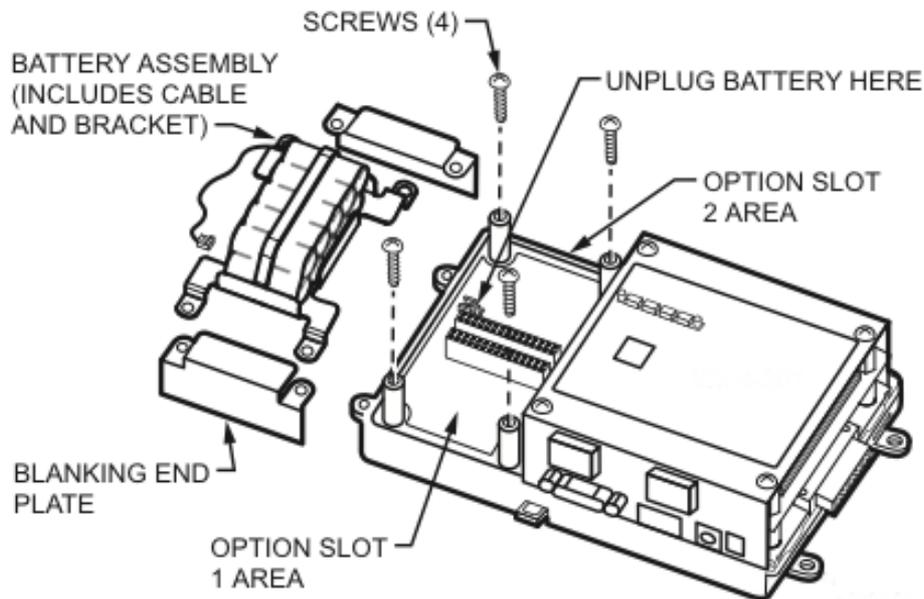
4. Remove the blanking end plate for the slot in which you plan to install the card.
